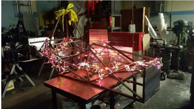
We have nearly completed the frame. The only parts left are to fabricate the steering supports and do the last of the finish welding before the structure will be finalized. Thank you to Fitz-Thors Engineering for their help in finishing our floor pans. As a result, we are now ready to begin drilling holes in the bottom of the frame to attach the floor which will happen after break.
