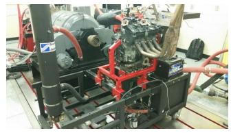
For the engine, we have recently finished the dynamometer stand. Our water-brake dynamometer uses water to resist the engine, allowing us to measure the torque. Knowing the torque output of the engine allows for more precise tuning which will contribute to our success at the competition in May. Before the end of the semester, we plan on completing and installing the
